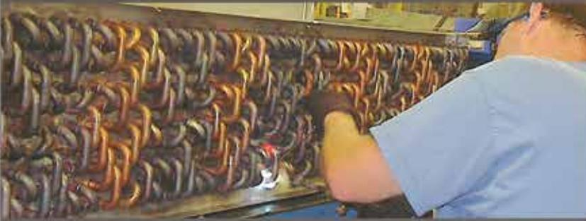
*Our reliable, hand-brazing process with silver bearing alloys is highly effective—ensuring that the coils you order from Precision will outlast most competitors.*
